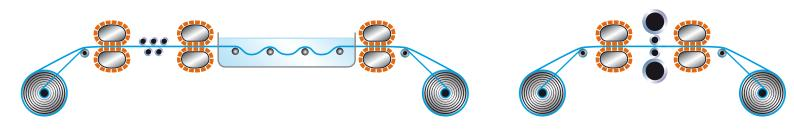
Umlauf Bridles have made a number of processes possible that used to be considered unfeasible for a long time, for example, rolling with a controlled pressure-tension ratio or continuous stretch-leveling. Also leveling several slit coils at the same time in slitting lines is something no one else can do."
