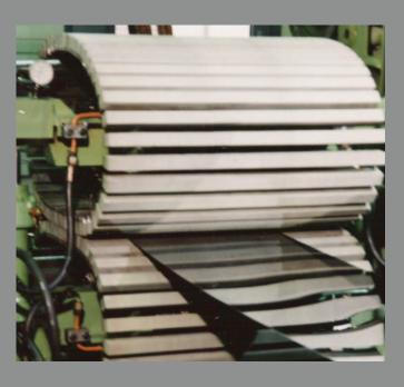
Umlauf Bridles increase and decrease strip tension as required – at virtually any position along the production chain, from the cold rolling mill down to the finishing facilities and in service centers.
