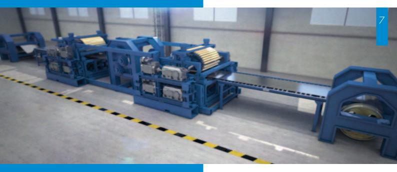
Ahead of a recoiler, a single Umlauf Bridle adjusts the strip tension and aligns the edge of the winding strip so as to produce perfect straight-edge coils.
